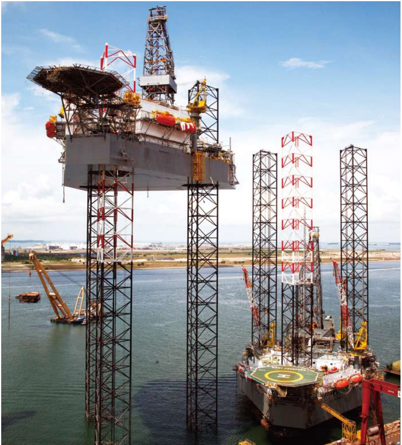
Keppel FELS has secured a third KFELS Super B Class Bigfoot contract from Transocean. This design is an enhancement of the KFELS Super B Class jack-up (shown here)
